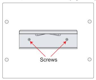
**Step 2:** Insert the top of the DIN-Rail into the Step 3: The DIN-Rail attachment unit will slot just below the stiff metal spring.
