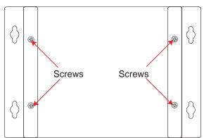
Step 2: Use two screws per side to attach the V2101 to a wall or cabinet.
