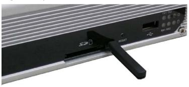
**Step 2:** After removing the cover, insert the SD memory card into the slot.
