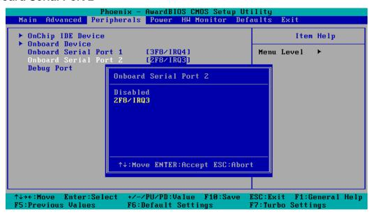
This function allows you to enable/disable serial port 2 communication. The V2101 computer will automatically distribute the IRQ value for serial port 2 as the default value. If you wish to disable, select **Disabled**.
