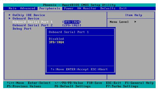
This function allows you to enable/disable serial port 1 communication. The V2101 computer will automatically distribute the IRQ value for serial port 1 as the default value. If you wish to disable, select **Disabled**.
