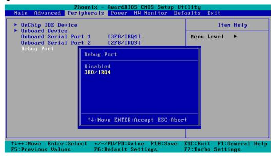
This function allows you to enable/disable the debug port communication. The V2101 computer will automatically distribute the IRQ value for the debug port as the default value. If you wish to disable, select **Disabled**. This port is only for engineers who are debugging programs.
